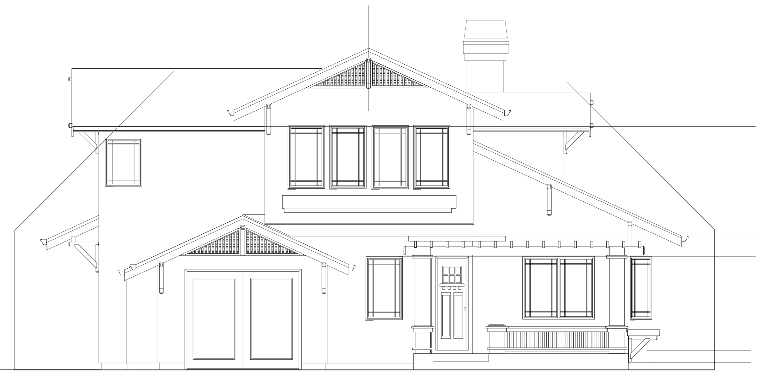
2 Elevation @ Front (North) Scale 1/4" to 1'-0"
